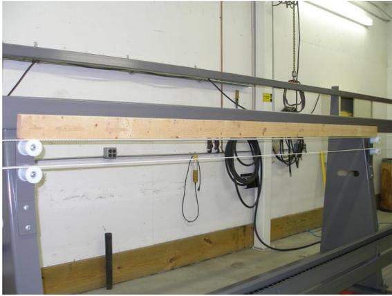
Drive Belt Tensioning – Board location
