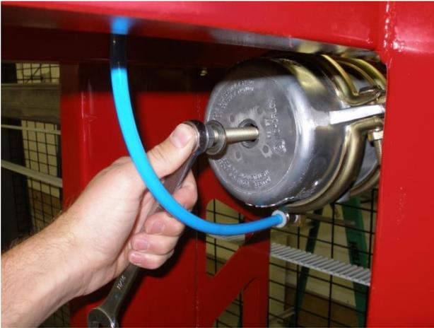
Turning release tool clockwise
