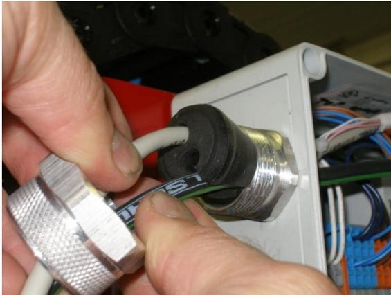
Ethernet Cable routing – Gantry Enclosure
