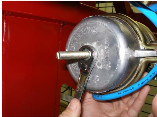
Tighten nut until spring is compressed
